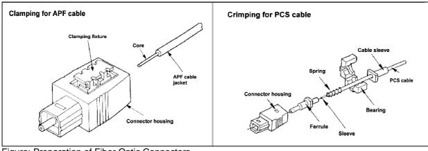
Figure: Preparation of Fiber Optic Connectors
