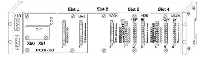
FOX-20 Basic Module with Four Analog Inputs, Four Analog Outputs, Eight Digital Inputs, Eight Digital Outputs
