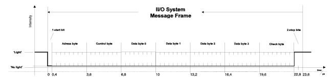
Figure 2: Message Structure of II/O-System
