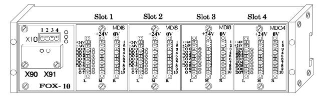
FOX-10 Basic Module Fitted with Four Input/Output Modules
