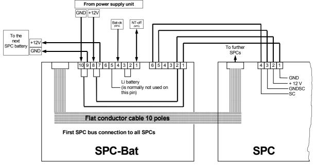
The signals nominated NPS are only used if an NPS power supply unit is available. Bat-Ok can only be read before the first SPC. The power supply unit is disabled before the first SPC (via software handshake internally in the DP-RAM).
